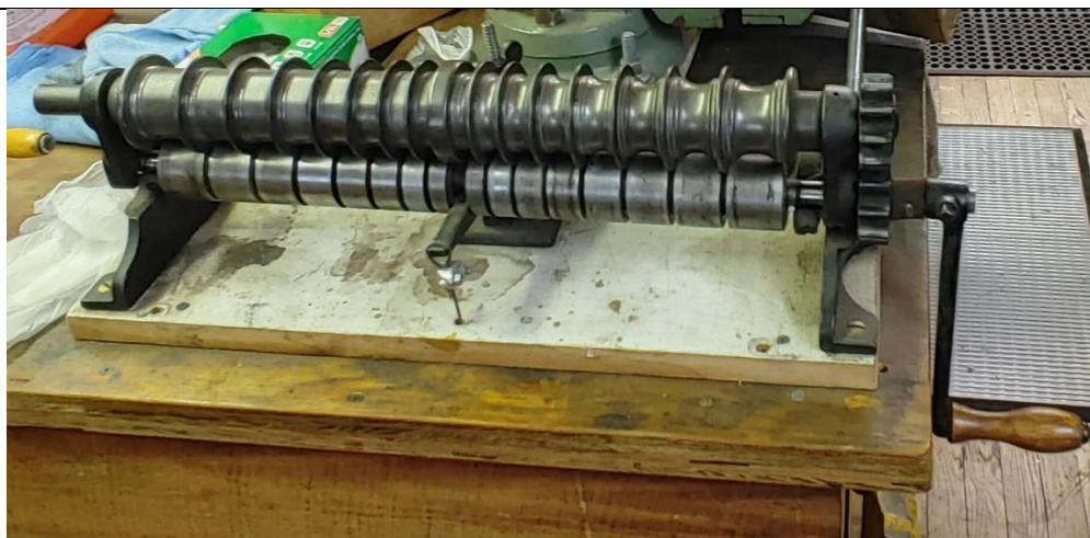
This 1867 C.C. Bellows Hand Crank Leather Creaser is used to mark where stitches go on leather straps and belts.
